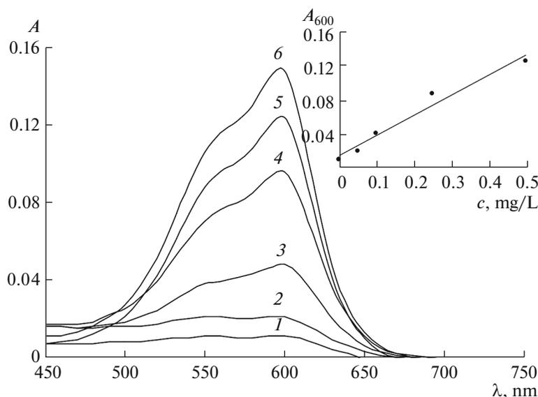
**Fig. 1.** Absorption spectra of Crystal Violet immobilized in a polymethacrylate matrix after contact with a solution of thiocyanate ions in the presence of bromate. Concentrations:  $\text{SCN}^-$  (1) 0, (2) 0.05, (3) 0.10, (4) 0.25, (5) 0.50, and (6) 1.00 mg/L;  $\text{BrO}_3^-$ ,  $3.0 \times 10^{-4}$  M; HCl, 0.3 M ( $a_{\text{CV}} = 0.08$  mg/g,  $t_{\text{contact}} = 3$  min,  $n = 3$ ,  $P = 0.95$ ). Inset: concentration dependence for thiocyanate at  $\lambda = 600$  nm.
